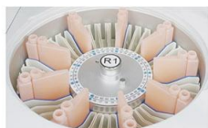
Reagent Tray 2~8°C cooling for 24 hours.
