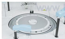
Reaction Tray 37±0.1°C, real-time monitor.
